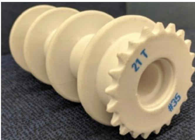
The maximum torque on the motor/gearing combination is approximately 60 ft./lbs. and it can stall this with no apparent ill effect.
